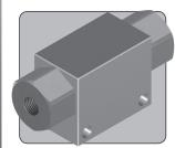
The SV50 is a 1/2" nominal bore shuttle valve. The valve will sense the higher of two pressures and send this pressure to the outlet port.
